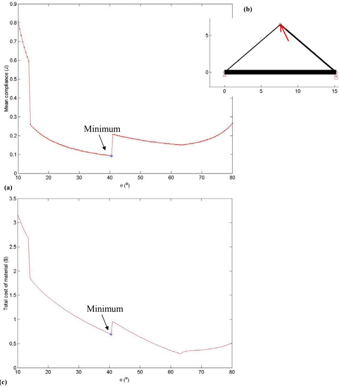
**Fig. 12 Example 3 with  $L = 10m, F = -100 N, n = 0.5$  (a) Stiffness measure,  $MC$  (b) Optimum truss where line-widths indicate relative proportions of cross-section on a scale of 1-10 with 10 showing the maximum width (c) Cost of material. (a) and (c) are plotted as a function of the geometric variable,  $\theta$ .**
