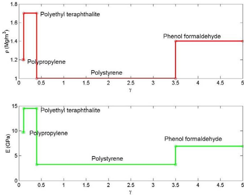
**Fig. 9 Properties relevant to stiffness optimization from the best *polymer* materials selected for each value of  $\gamma$ . Mean values are shown instead of the min/max values for each property.**
