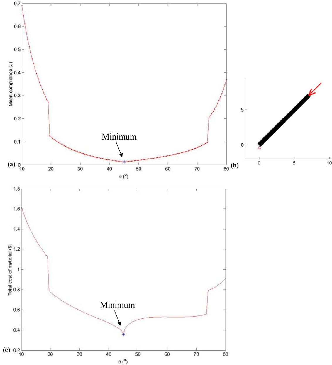
**Fig. 11** Example 1 with  $L = 10\text{ m}$ ,  $F = 100\text{ N}$ ,  $n = -1$  (a) Stiffness measure,  $MC$  (b) Optimum truss where line-widths indicate relative proportions of cross-section on a scale of 1-10 with 10 showing the maximum width (c) Cost of material. (a) and (c) are plotted as a function of the geometric variable,  $\theta$ .
