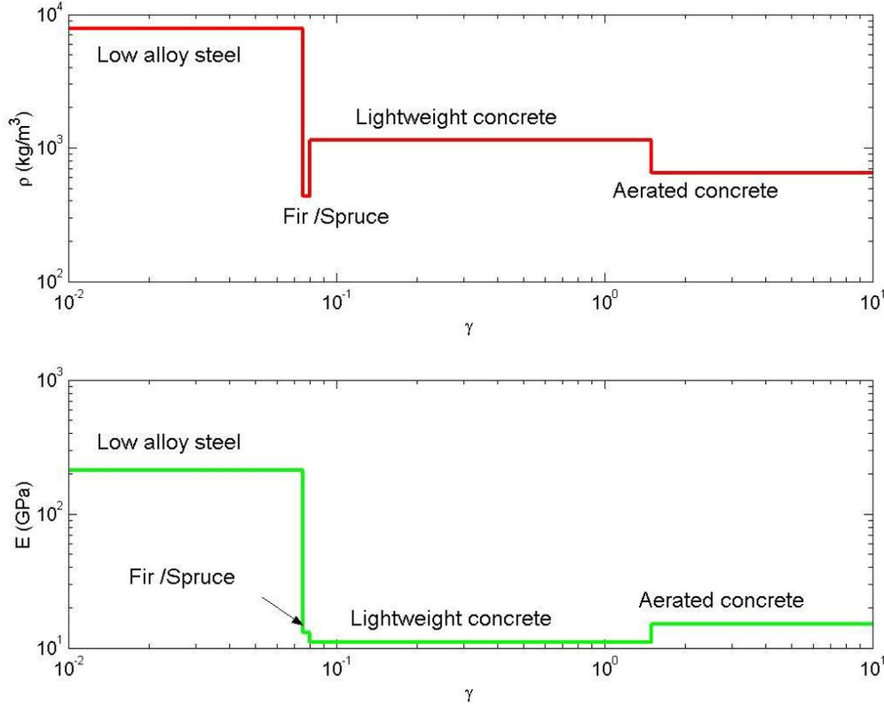
**Fig. 8 Properties relevant to stiffness optimization from the best materials selected for each value of  $\gamma$ . Mean values are shown instead of the min/max values for each property.**
