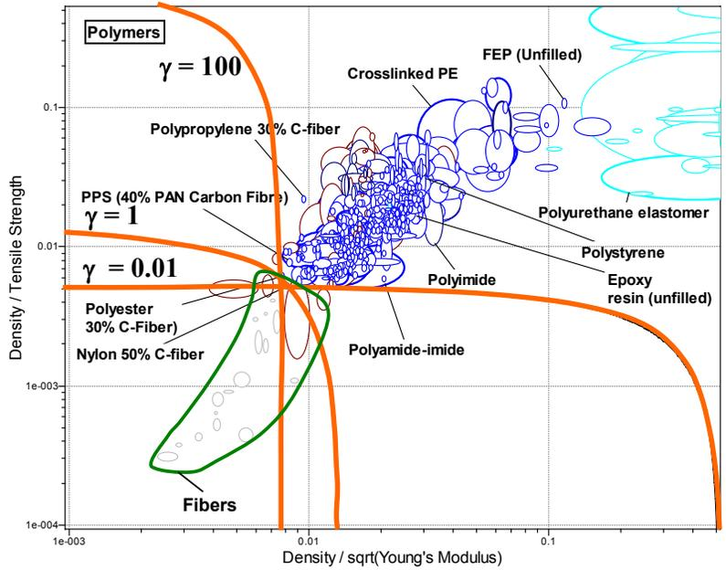
Fig. 5 Material selection for trusses considering only polymers. Fiber reinforced polymers appear to be the best because cost is not a criterion. Fibers themselves, enclosed in the green envelope, are ignored.
