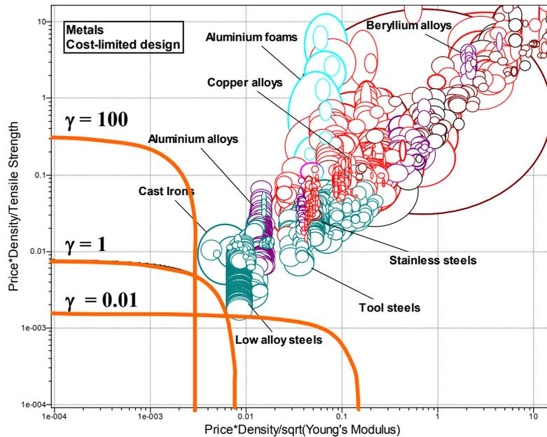
Fig. 4 Material selection for trusses considering only metals but cost included. Low alloy steels and cast irons now emerge as the best candidates.
