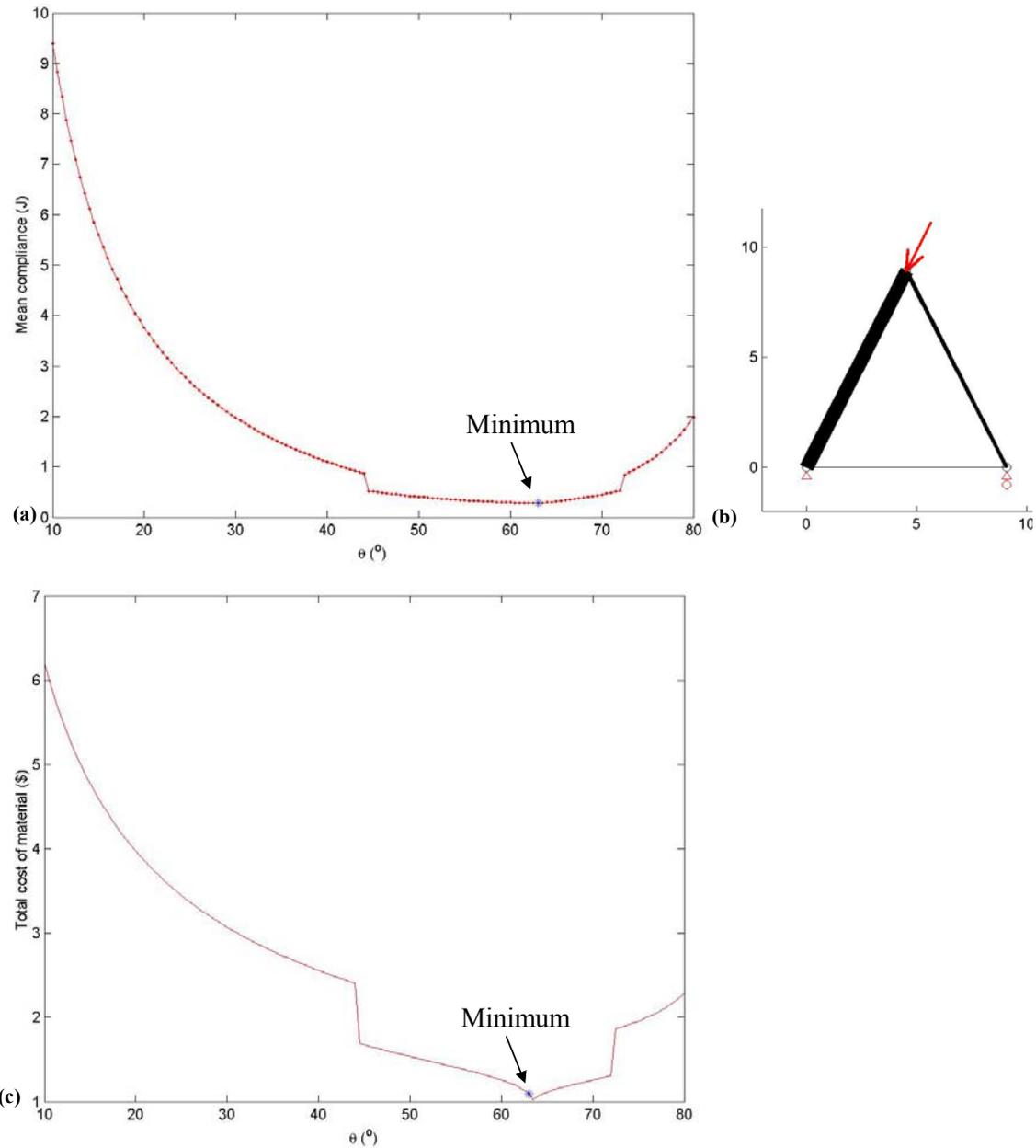
**Fig. 10** Example 1 with  $L = 10\text{ m}$ ,  $F = 1000\text{ N}$ ,  $n = -0.5$  (a) Stiffness measure,  $MC$  (b) Optimum truss where line-widths indicate relative proportions of cross-section on a scale of 1-10 with 10 showing the maximum width (c) Cost of material. (a) and (c) are plotted as a function of the geometric variable,  $\theta$ .
