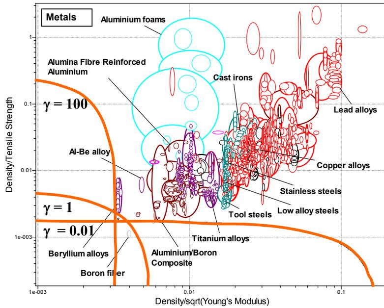
Fig. 3 Material selection for trusses considering only metals. Since price is not included, expensive alloys and fiber composites turn out to be the most suitable materials to minimize the mass.
