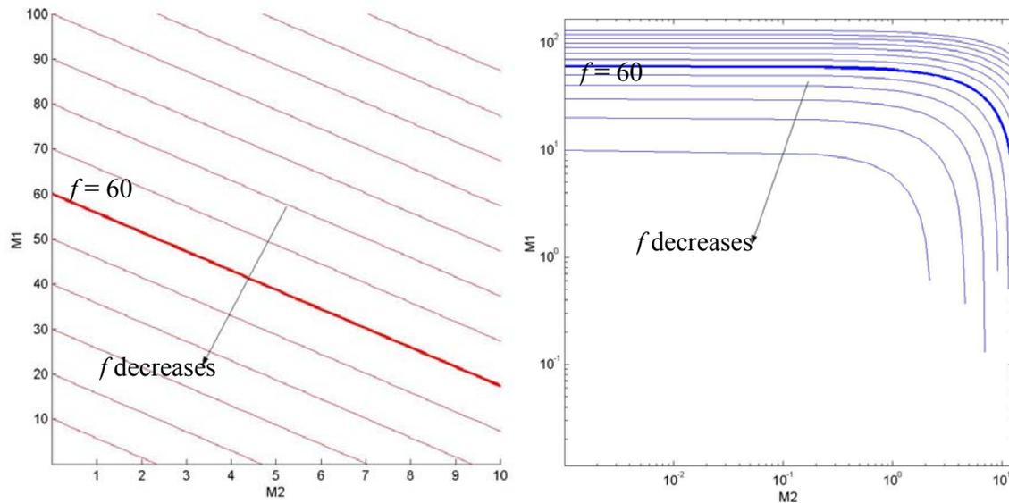
**Fig. 2 Visualizing the minimization of a performance measure  $f$  that is a linear combination of two material indices,  $M_1$  and  $M_2$  for a given ratio of their weights. (a) linear plot (b) log-log plot**
