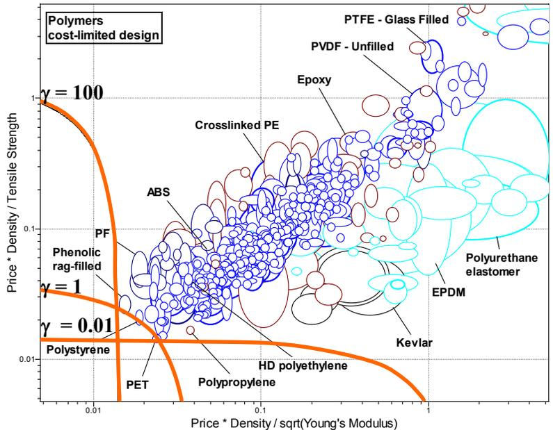
Fig. 6 Material selection for trusses considering only polymers. With cost included, polypropylene, polystyrene, etc., emerge as the most suitable materials.
