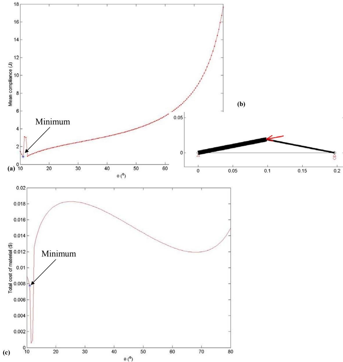
**Fig. 13** Example 4 with  $L = 0.1m, F = 1000N, n = -5$  (a) Stiffness measure,  $MC$  (b) Optimum truss where line-widths indicate relative proportions of cross-section on a scale of 1-10 with 10 showing the maximum width (c) Cost of material. (a) and (c) are plotted as a function of the geometric variable,  $\theta$ .
