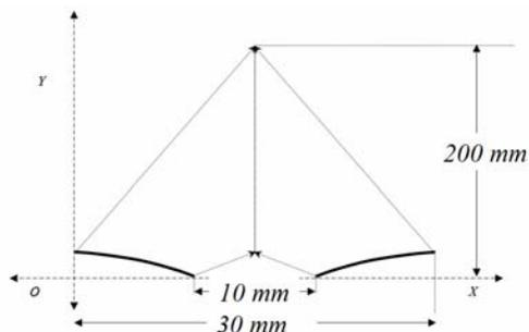
Figure 5: Quantitative details of the desired motion of the two cameras (thick circular arcs) mounted on the mechanisms that should collapse into a tube of diameter 15 mm.
