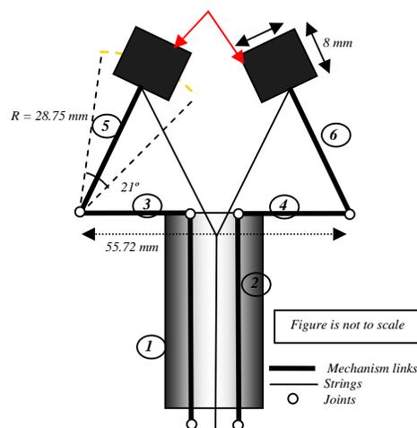
Figure 6: Schematic of the mechanism with the cameras.
