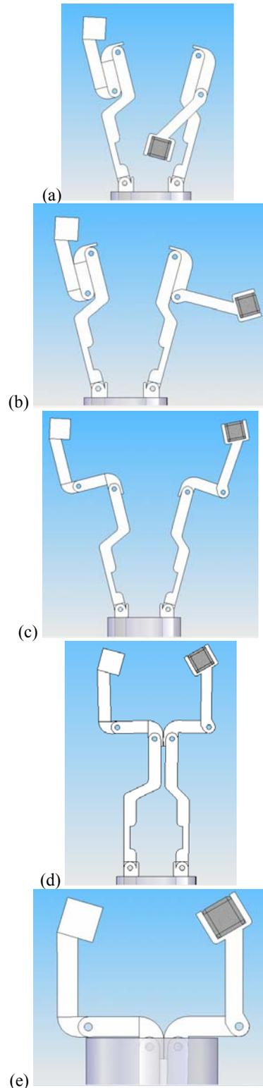
Figure 9: Deployment steps of the mechanism. (a) Pushing it out of the tube takes the two arms apart to enable them to unfold by releasing their torsional springs, (b) Unfolding of the right arm, (c) Unfolding of both the arms, (d) pulling both the arms into their required positions, and (e) pulling the whole assembly to rest against the edge of the tube.
