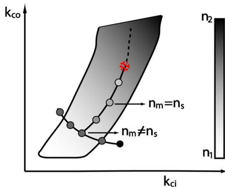
**Fig. 10 Redesign by using multiple parameter curves. One of the curves is selected for redesign but it does not result in matched values of  $n_m$  and  $n_s$ . Hence, an alternate parameter curve is pursued from within the feasible map to obtain a feasible mechanism. The red STOP sign on the second parametric curve indicates that a particular manufacturing process limit has been reached because of the change in the corresponding parameter.**
