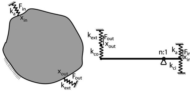
Fig. 5 The variables involved in the SL model of a single-input-single-output compliant mechanism
