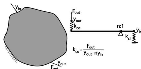
**Fig. 4 The second load case used to find the output side spring stiffness  $k_{co}$  of the SL model**
