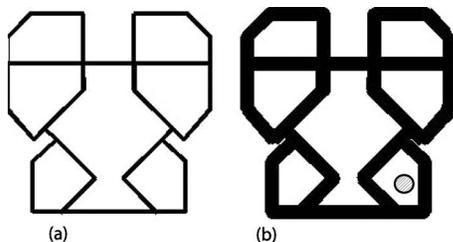
**Fig. 11 Redesigning a mechanism by changing its in-plane width: (a) the mechanism as it is in the database and (b) redesigned mechanism with increased width, which is limited by the tool diameter shown as a hatched circle**
