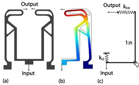
**Fig. 1 Spring-leverage model: (a) a compliant gripper, (b) its symmetric half used in deformation analysis, and (c) its representation as a lever with geometric amplification factor  $n$ , the input-side spring stiffness  $k_{ci}$ , and the output side spring stiffness  $k_{co}$**
