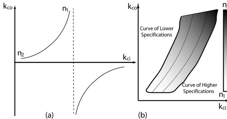
Fig. 6 Drawing the feasible map on the selection map: (a) the points on the curve are generated for lower bounds of the specification variables but with different values of *n*; only the part of the curve corresponding to the positive values of  $k_{ci}$  and  $k_{co}$  is considered and (b) the feasible map is bounded by the curves corresponding to the upper and lower specification variables and is filled with a gray color scale based on the value of *n*
