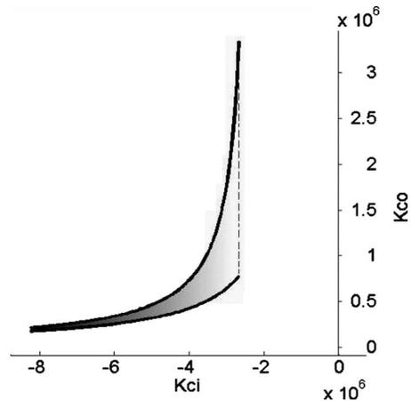
Fig. 14 The feasible map is bound by the curves representing the lower and upper bounds on specification variables
