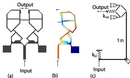
**Fig. 2 SL model to match the kinematic behavior: (a) a compliant gripper, (b) its symmetric half used in deformation analysis, and (c) a leveraging mechanism to revert the direction of motion from input to output in the SL model to match the output direction in the gripper**
