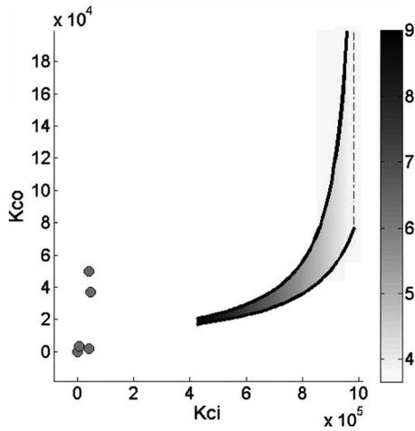
Fig. 15 The feasible map for the modified specifications shown in Table 1 with output load reduced to 10 N. The dots show the mechanisms that are closest to the feasible map.
