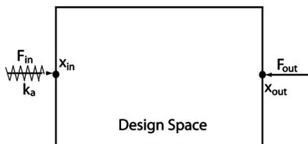
Fig. 13 Design problem of a compliant mechanism to amplify the motion of a piezoelectric actuator at the output
