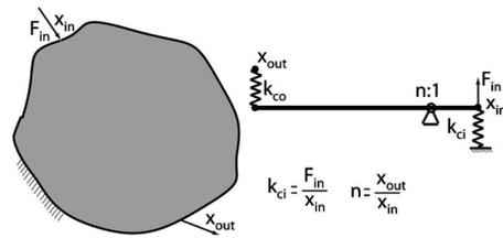
**Fig. 3 The first load case used to find the input-side stiffness  $k_{ci}$  and the inherent geometric amplification factor  $n$  of the SL model**
