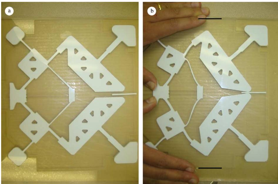
Fig. 15. A polypropylene prototype of the grasp and pull gripper design in its original (left) and deformed (right) configurations.
