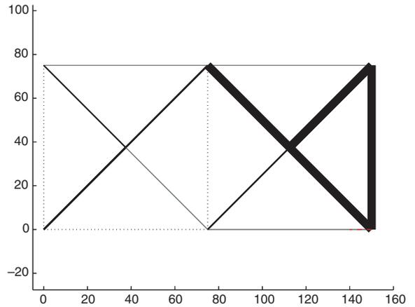
Fig. 27. The design for a mechanical frequency doubler obtained from the synthesis procedure. The axes are marked in mm.
