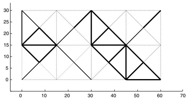
Fig. 14. The grasp and pull gripper design obtained from the solution procedure. The axes are marked in mm.
