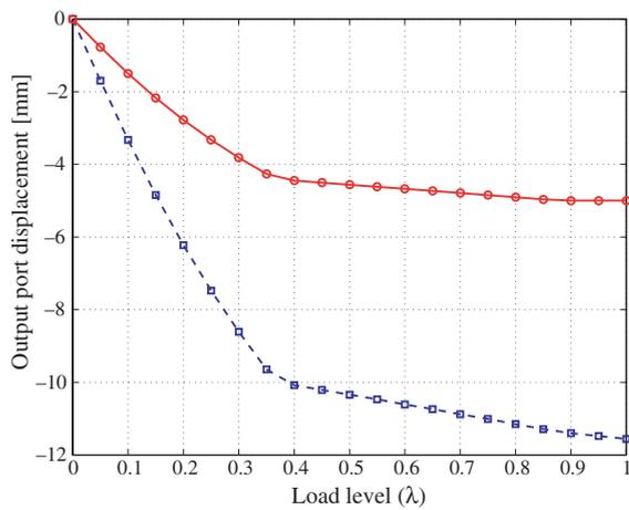
Fig. 25. The  $X$  displacement (dashed black curve with squares, blue) and the  $Y$  displacement (solid gray red curve with circles, red) of the output port for the final design. (For interpretation of the references in colour in this figure legend, the reader is referred to the web version of this article.)
