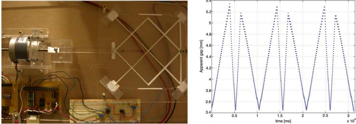
Fig. 32. Experimental setup to test a polypropylene prototype of the mechanical frequency doubler (left) and output displacement corresponding to three input cycles (right).
