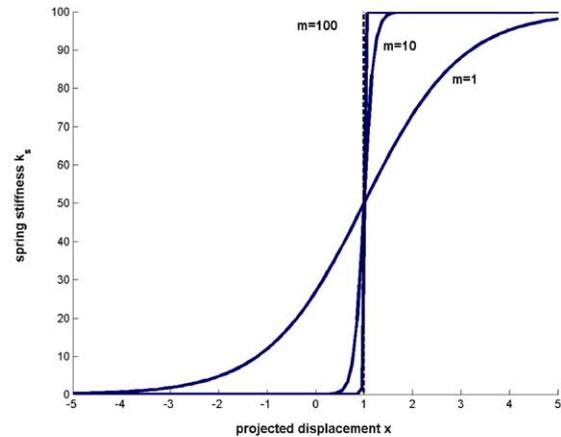
Fig. 6. Smoothed modeling of contact for small deflections: (a) a nonlinear spring with variable stiffness models the contact, (b) parametric regularized contact stiffness function.
