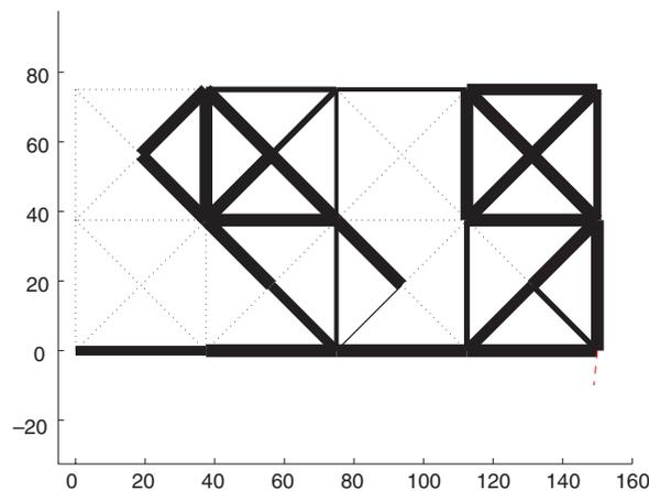
Fig. 20. The displacement delimited gripper design obtained from the sequential optimization procedure. The axes are marked in mm.
