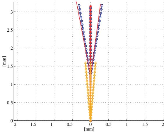
Fig. 12. The path of the output port of the OR gate design for different load conditions as predicted by nonlinear FEA using ABAQUS®.
