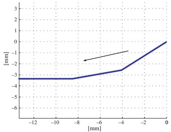
Fig. 18. The simulated path for the output port of the grasp and pull gripper obtained from nonlinear FEA using ABAQUS.
