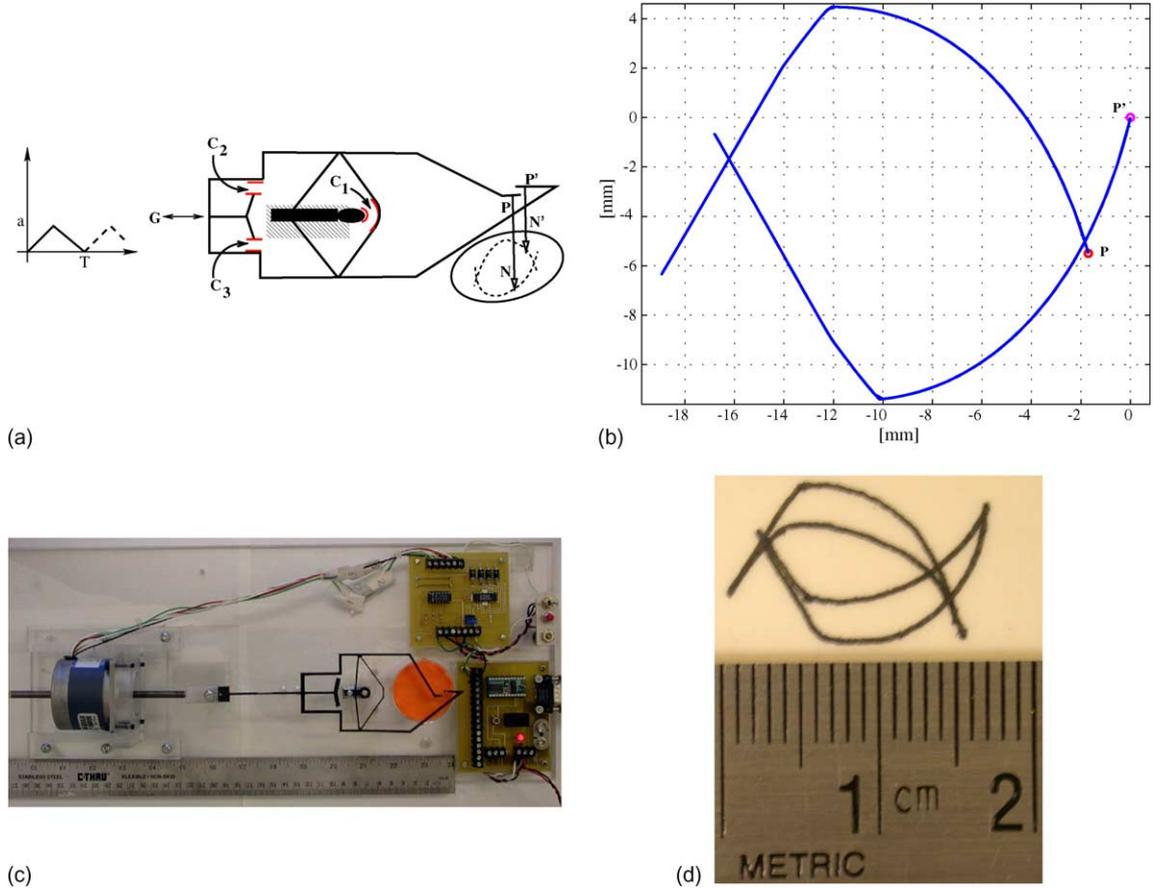
Fig. 3. A CCM with three contacts to generate a pair of sharply curved arches: (a) schematic, (b) the simulated curves without the output load at the points, (c) polypropylene prototype driven by a stepper motor, (d) curves obtained from the experiment.
