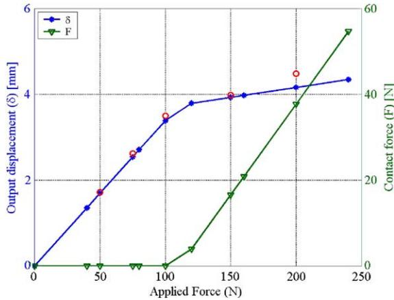
Fig. 16. Performance characteristics of the grasp and pull gripper.
