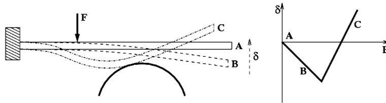
Fig. 1. Nonsmooth force–deflection behavior from a cantilever beam contacting a rigid surface.
