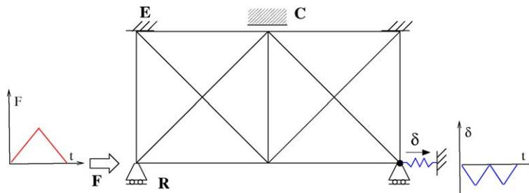
Fig. 26. Schematic of the problem formulation for the mechanical frequency doubler. The output node displacement ( $\delta$ ) is positive in the direction shown by the arrow.
