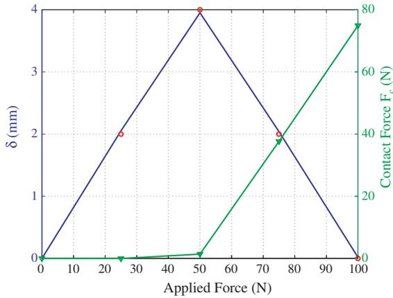
Fig. 29. Performance characteristics of the mechanical frequency doubler (one-half of the input cycle).
