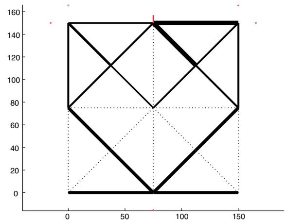
Fig. 9. The design for a mechanical OR gate obtained from the solution procedure. The axes are marked in mm.
