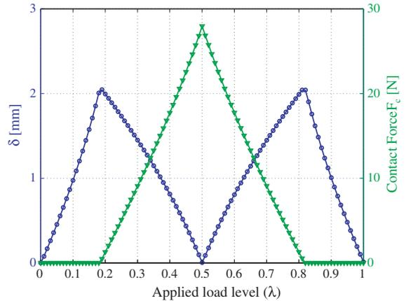
Fig. 30. Performance characteristics of the modified mechanical frequency doubler obtained from geometrically nonlinear FEA in ABAQUS.
