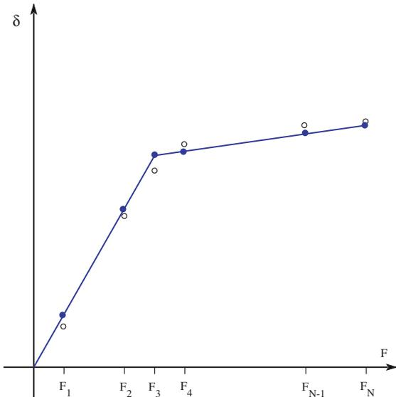
Fig. 7. Nonsmooth response specification for CCMs synthesis. The circles indicate the design data points, while the dots indicate the response of an actual trial mechanism.
