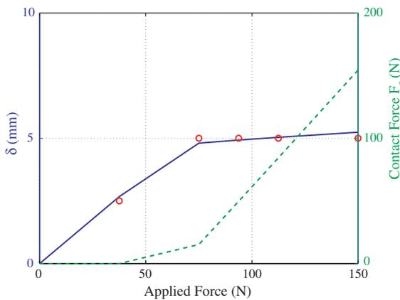
Fig. 22. Performance characteristics of the displacement delimited gripper.
