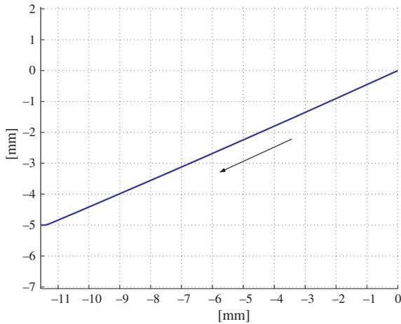
Fig. 24. The path for the output port of the displacement delimited gripper as simulated by nonlinear FEA using ABAQUS.
