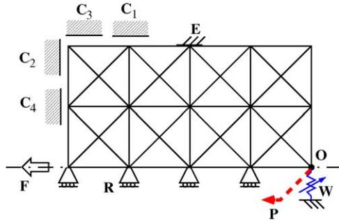
Fig. 19. Schematic of the problem specification for the synthesis of a displacement delimited gripper.
