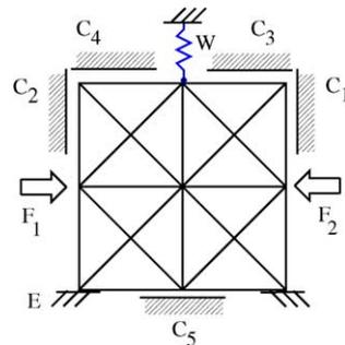
Fig. 8. Schematic of the problem specification for the synthesis of a mechanical OR gate.
