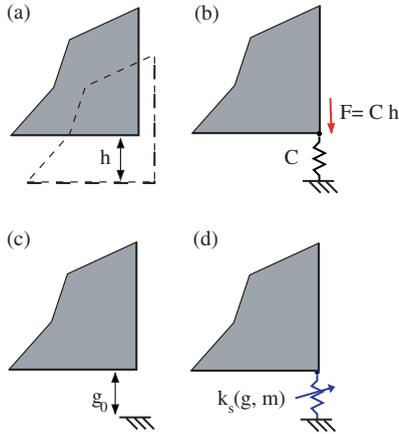
Fig. 5. A nonlinear spring can be used to model unilateral contact displacement boundary condition. Panels (a) and (b) show the penalty approach to model specified displacement ( $h$ ) boundary conditions at a node in FEM. Panels (c) and (d) show how that idea can be extended to model unilateral contact boundary conditions using a nonlinear spring.
