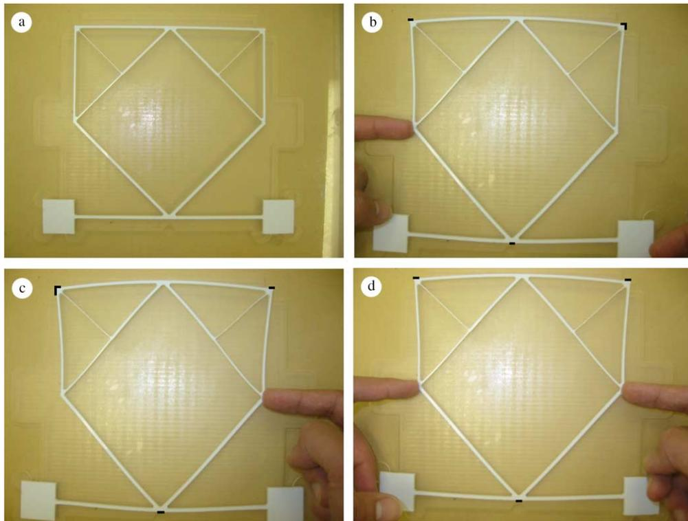
Fig. 10. A prototype of the symmetric design milled from polypropylene is shown in (a). The deformed configurations under load cases 1, 2 and 1 + 2 are shown in (b)–(d) respectively.
