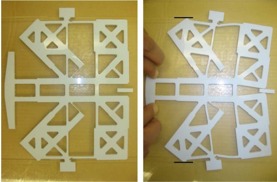
Fig. 21. A polypropylene prototype is shown in the original configuration (left) and in the actuated configuration (right).
