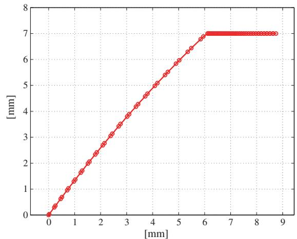
Fig. 31. The path of the contact node for the modified mechanical frequency doubler as predicted by geometrically nonlinear FEA in ABAQUS.
