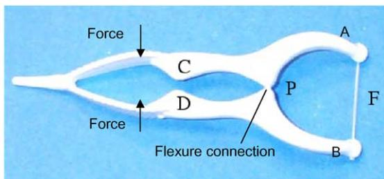
Fig. 2. Dental floss tool as an example of a CCM that undergoes an abrupt change in stiffness.
