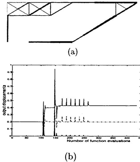
Fig. 10 Two-point force-deflection synthesis of a compliant crimpers (a) optimal topology for design case III (b) convergence history
