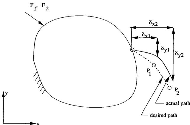
Fig. 12 Design specifications for prescribed curved output path
