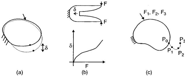
**Fig. 1 Synthesis capabilities using nonlinear finite element analysis (a) quantitative accuracy for large deformations (b) prescribed nonlinear force-deflection specifications (c) curved output paths**
