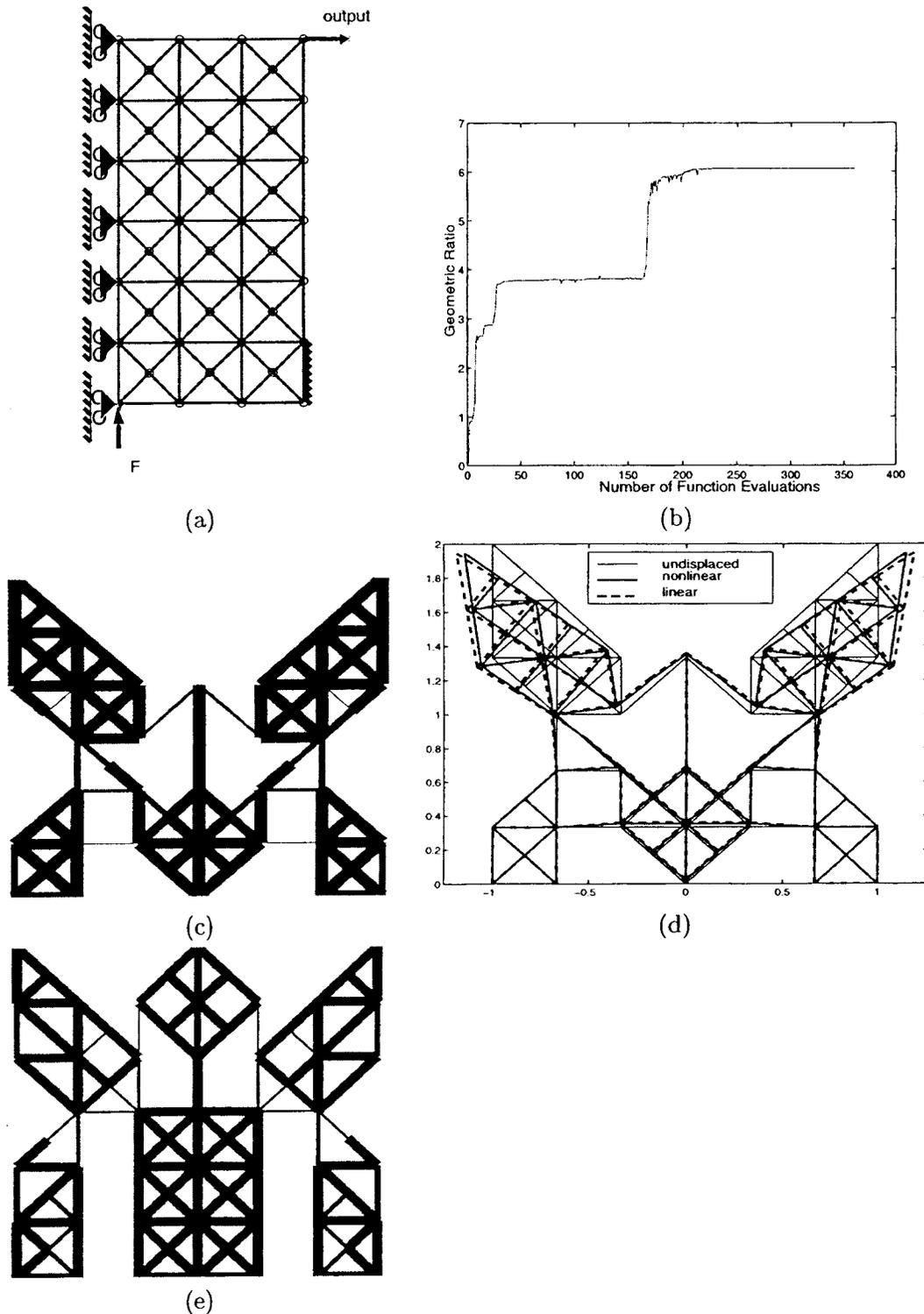
**Fig. 6 Topological synthesis of a micro displacement amplifier. (a) Design specifications;  $F=500 \mu\text{N}$  (b) convergence history for topology optimization (c) full section design of the displacement amplifier (d) displaced profile; geometric advantage is 6.2 (e) optimal topology for  $F=100 \mu\text{N}$ .**
