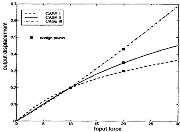
Fig. 11 Comparison of nonlinear force-deflection characteristics of the crimpers designs (Figs. 8–10)
