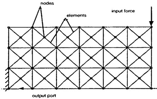
**Fig. 7 Design domain for two-point compliant crimper force-deflection synthesis**
