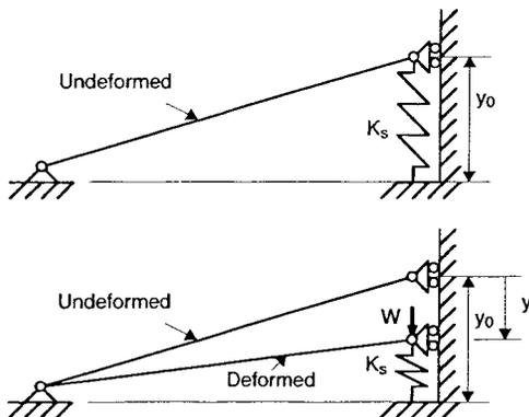
**Fig. 2 A bar with geometrically nonlinear deformation**
