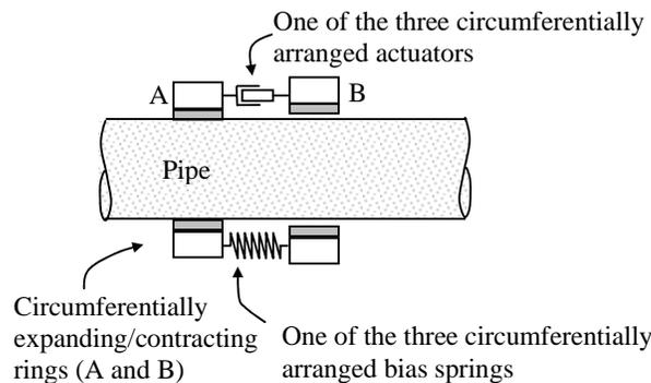
**Figure 2.** Schematic illustration of a clamp-and-push concept of a pipe-crawler.
