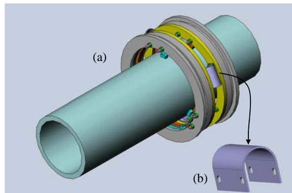
**Figure 9.** The solid model of the crawling device with the clamping rings and three SMA U-shapes strips. The spring steel bias spring strips are not shown in this picture.
