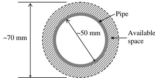
**Figure 1.** Spatial specifications of an external pipe-crawler. Only the hatched annular space is available for the crawler.
