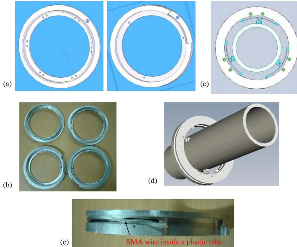
**Figure 8.** Housing and assembly for the clamping ring. (a) two halves of the housing, (b) two pairs of aluminium housings made using CNC milling, (c) solid model of the assembled clamping ring, and (d) the clamping ring on the pipe.
