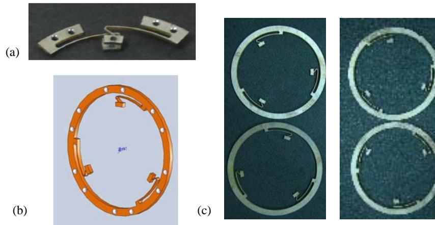
**Figure 7.** (a) A pair of spring steel compliant segments soldered together. This pair is the main element of the compliant radially expanding mechanism, (b) solid model of a ring with three compliant segments, and (c) four spring steel rings that help create two clamping ring upon soldering of two rings at the interior clamping points.
