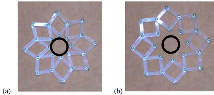
**Figure 3.** Radially deployable Hoberman's linkage. (a) clamping a pipe externally, (b) releasing the clamp.
