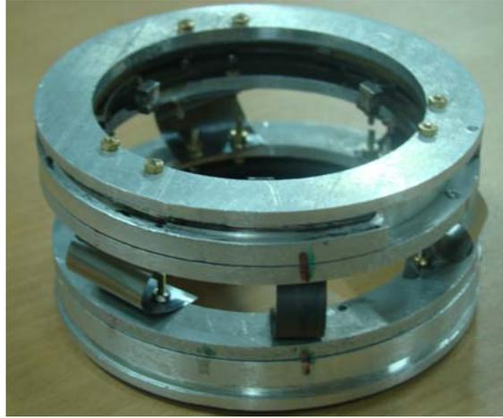
**Figure 10.** The complete prototype of the crawling device.
