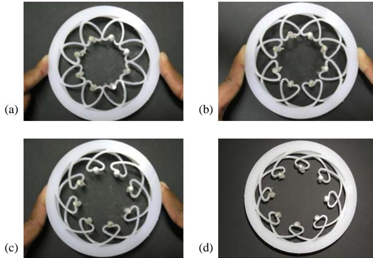
**Figure 5.** Circumferentially actuated radially deployable compliant mechanism prototype using polypropylene. It consists of two identical layers attached to each other at the innermost points and arranged one over the other. As the rings rotate relative to each other, the attachment points move radially inward or outward. Configuration in (d) is the undeformed while the one in (a) has the most deformation; (b) and (c) are intermediate configurations.
