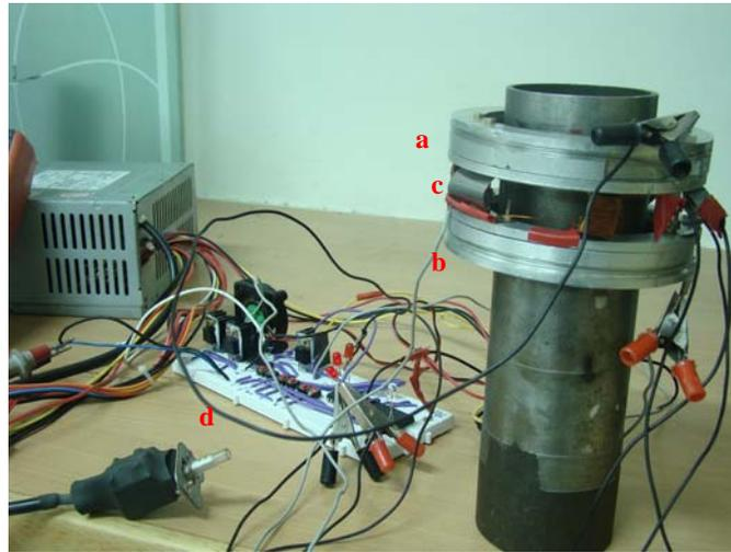
**Figure 11.** Test set-up of the crawling device. (a) clamping ring 1; (b) clamping ring 2; (c) SMA strip for linear actuation; and (d) control circuit to effect cyclical triggering of the three actuators: two SMA wires and one set of SMA strips.
