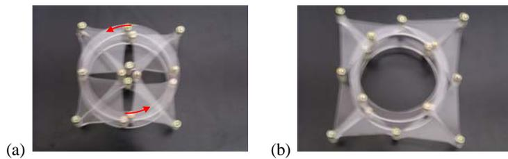
**Figure 4.** Circumferentially actuated radially deployable linkage from [14]. (a) completely closed configuration, (b) completely open configuration.
