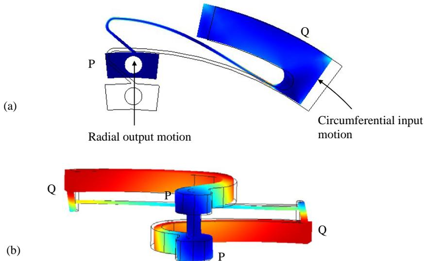
**Figure 6.** (a) A single compliant element that transforms a circumferential input motion to an amplified radial motion. The filled configuration is the deformed configuration obtained using finite element analysis. (b) Two compliant segments attached to each other and arranged one over the other. Note that the attachment of two P portions automatically constrains the radial movement. By arranging several such pairs along a circle ensures that Q portions move only circumferentially.
