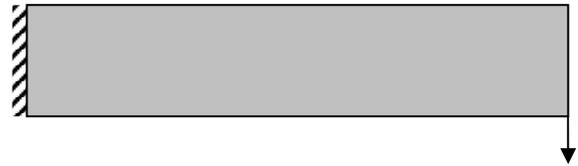
**Figure 6.** Design domain for the cantilever problem with boundary conditions
